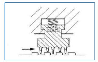
Figure 5 Spring Loaded Vernier Labyrinth Seal
