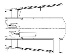
Figure 25. F-class axial diffuser
