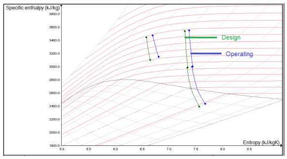
Figure 6.1: h-s diagram of turbines for unit - 1
