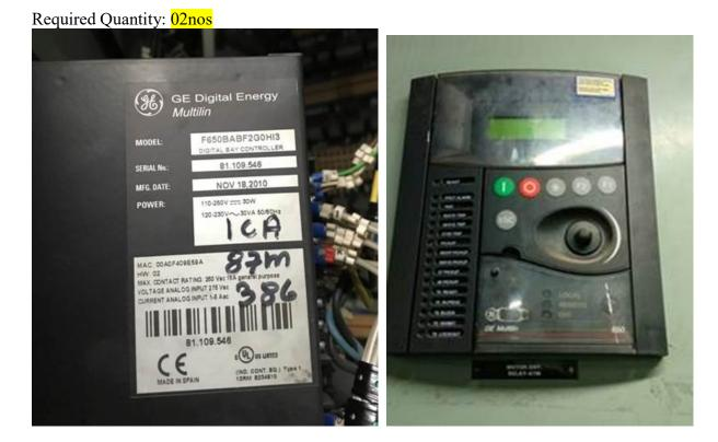
5. GE Multilin 650 Relay for Under Voltage/No Voltage Protection (6.6KV System) Protection Against: Under Voltage/No Voltage Fault (27/27N) Required: 02nos
