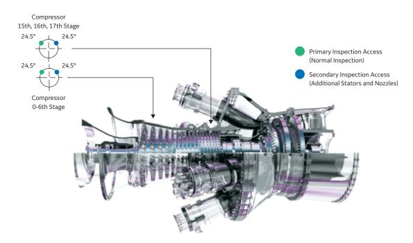
Figure E-5. 6FA.03 Borescope port locations
