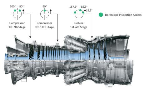
Figure E-4. 7HA.01 gas turbine borescope inspection access locations
