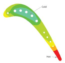
Figure 16. Second stage bucket transient temperature distribution
