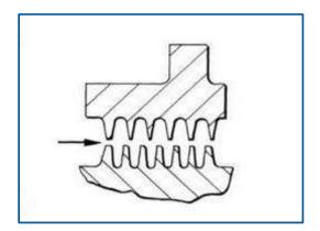
**Figure 4 Vernier Labyrinth Seal**
