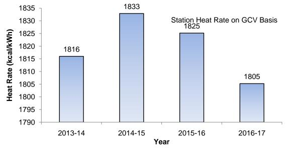
Figure 1.3: Plant Heat Rate
