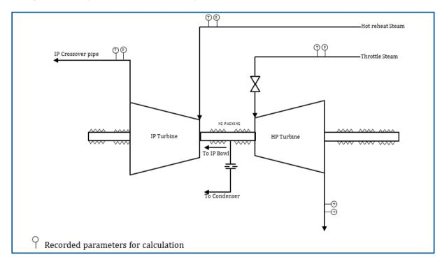
Figure 7 Determining HP-IP Leakage (Temperature Inference Method)
