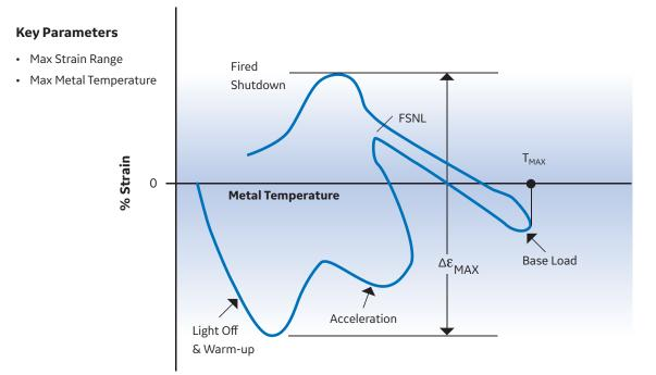
Figure 17. Representative Bucket low cycle fatigue (LCF)"
