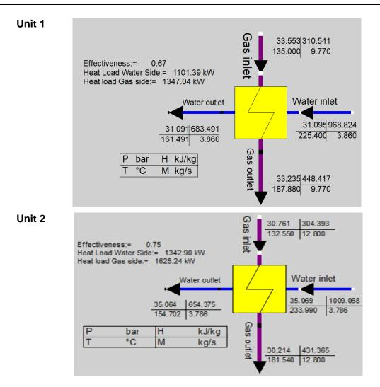
Figure 4.2: Performance heater Energy & Mass Balance
