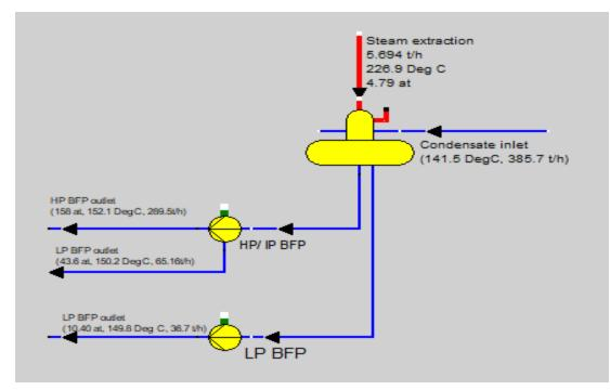
Figure 8.1: Process flow diagram of BFP
