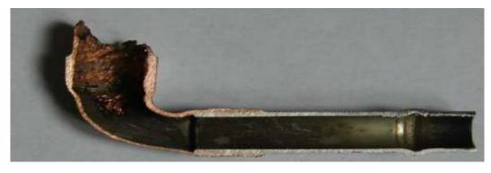
Figure 3: Cross section of eroded pipe removed from water cooled bus bar
