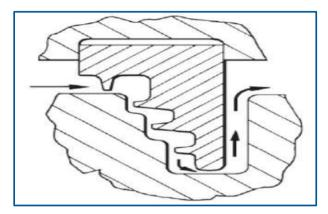
Figure 6 Labyrinth Glands with Axial and Radial Fins
