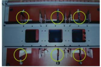
Figure 2 : Load bridge water-cooled bus ends (front side) without SCRs and capacitor installed
