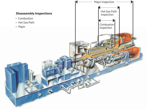
Figure 29. 7E.03 heavy-duty gas turbine – disassembly inspections
