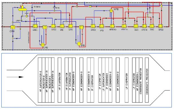
Figure 5.1: HRSG process flow and arrangement diagram
