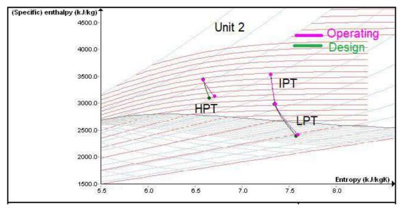
Figure 6.2: h-s diagram of turbines for unit -2
