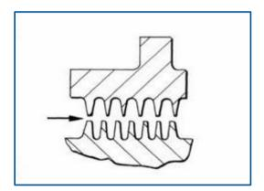
**Figure 4 Vernier Labyrinth Seal**
