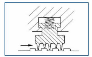
**Figure 5 Spring Loaded Vernier Labyrinth Seal**
