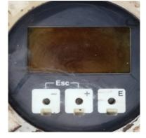
2 Flowmeter found to be Powering ON with rated Power supply
