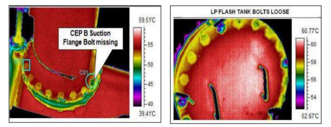
Figure 14 Infrared Thermography CEP Suction Flange Figure 13 LP Flash Tank
